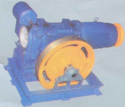
Lift drive unit with motorised worm speed reducers
